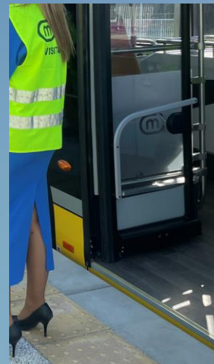
LEVEL ACCESS BETWEEN THE PLATFORM AND THE VEHICLE
